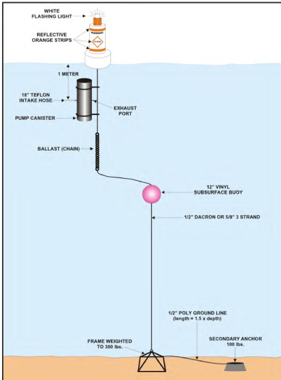
Figure 4. Moorings deployed to measure nearshore background water quality
