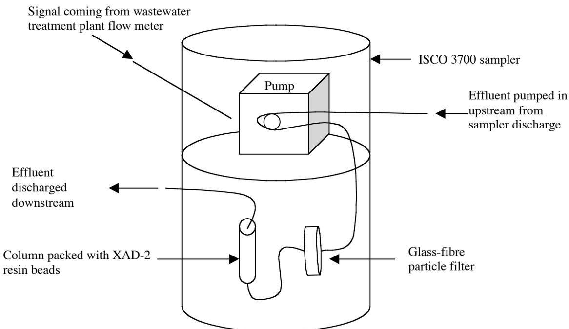
**Figure 3. Configuration of ISCO samplers for CCLEAN effluent and river sampling.****Table 2. Dates and volumes of effluent and river samples, 2006–2007.**
